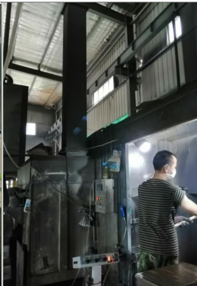
喷塑流水线手工喷枪及自带粉尘回收设施
